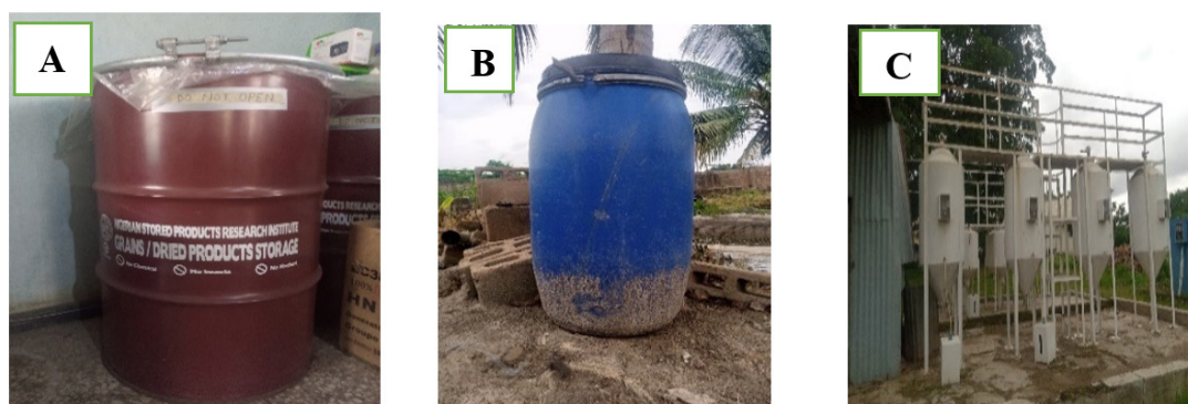
Figure 5: A: NSPRI's Hermetic Steel Drum, B: plastic hermetic rubber, C: Experimental Silo. Image taken by: N.F. Okparavero (Nigerian Stored Products Research Institute, NSPRI).
